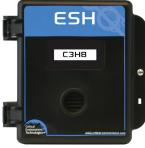
The ESH-A Remote Sensor offers flexible location monitoring of combustible or PID TVOC gases in non-hazardous, non-explosion rated, commercial and light industrial applications. It communicates with a controller or transmitter using current loop into a 100 ohm load or a voltage signal of 0.40 to 2 volts.
