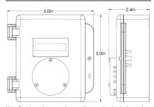
Note: Drawings above are shown with an optional splash guard. Without splash guard, thickness of unit is 2.1" (53 mm).
