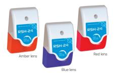
The Remote Strobe / Horn combines two alarm features, a visual and an audible into one compact, low profile device. It is powered by 24 VDC / VAC. The strobe and siren can be configured to activate together or each can activate separately from each other. It is recommended that this device be suitably mounted on a standard electrical box with conduit and protected from water ingress.
