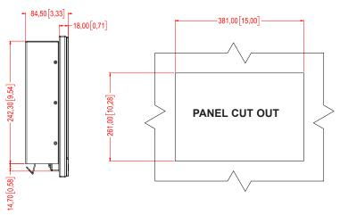
Dimensions might be shown with or without decimals and indicated as mm [inches]. Tolerance on drawings is +/- 1mm. For accurate measurements, check relevant DWG file.
