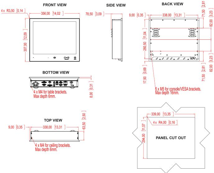
Dimensions might be shown with or without decimals and indicated as mm [inches]. Tolerance on drawings is +/- 1mm. For accurate measurements, check relevant DWG file.
