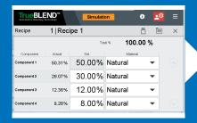
View and make changes to the active recipe Save and recall up to 3000 recipes and 4000 resin names in the
