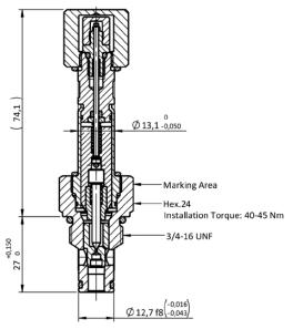
EVSC.34 valves are to be installed in cavity 3/4" 16 UNF with Ø 12,7 mm. Check the appropriate state and position of the seals supplied with the valve :
