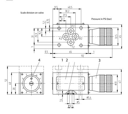
All stackable valves AM3-Q3- \* conform with ISO and CETOP specifications for mounting surface dimensions and for valves height 40 mm. Leakage between valve and mounting surface is prevented by the positive compression on their seats of 4 seals type OR 2037.
