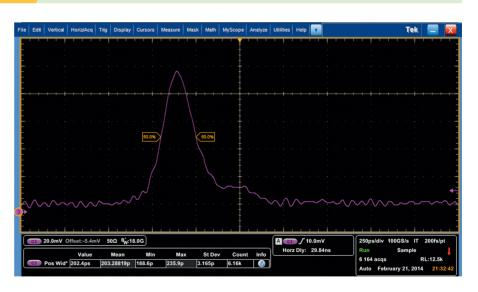
STA-01-6 model with pulse duration less than 190 ps
