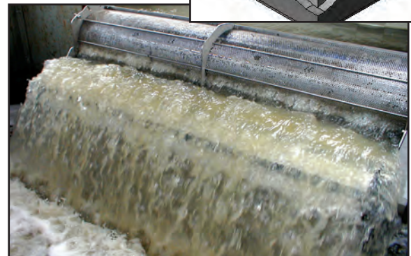
2 Stormscreens installed to screen storm overflows
