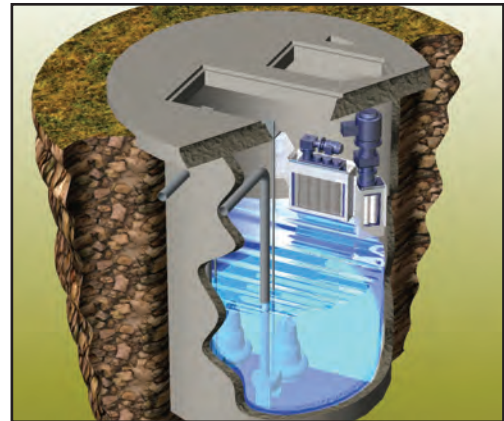
Discreen / Muncher combination for pump protection
