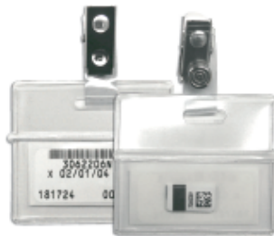
The Neutrak dosimeter packaged in a vinyl pouch specifically for neutron detection only
