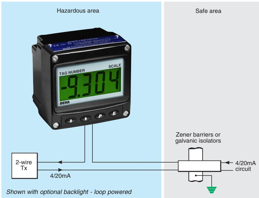
The **BA304G loop powered** 4/20mA indicator is a new field mounting instrument that supersedes the well established BA304C. It is electrically and mechanically compatible with the earlier model but has a much larger full 4 digit display and guaranteed performance between -40 and +70°C. Like its predecessor, the BA304G is housed in a robust IP66 enclosure which may be surface or pipe mounting.
