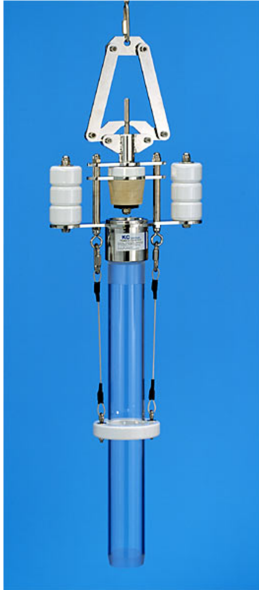
Kajak Sediment Sampler Model 13.030
