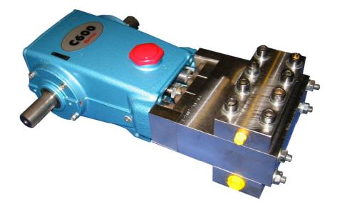
C600 pump is a triplex type positive displacement high pressure pump with spring operated suction and pressure valves. C600 pump consists of oil lubricated drive end and fluid end in contact with the pumped media. The body of the drive end is of casted alloy. Parts that come in contact with pumped media are of stainless steel (1.4401, AISI 316, or better from the corrosion point of view) and special plastics.
