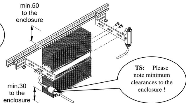
The brackets in zinc coated steel and fixing bolts illustrated above are included with the heater.
