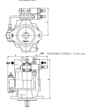
① = Regulation screw for max displacement. Adjustable range 50% to 100% of max displacement). In case of double pump the regulation screw is not always available, please contact our technical office.
