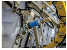
Thanks to highly accurate ultrasonic sensors and a control valve, we are able to achieve width variations of less than +/- 2 mm even on existing systems
