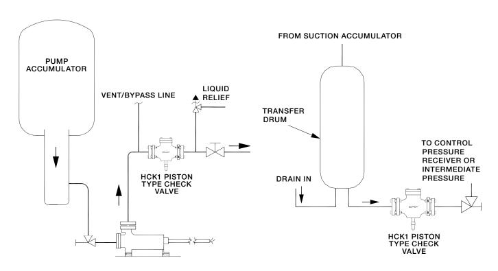
The above are schematic drawings of fictional refrigeration systems to show Hansen product applications in a system. These drawings should not be used for design or construction.
