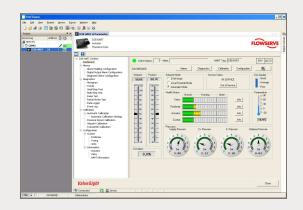
ValveSight monitors the health of the valve, actuator, positioner and control signal, displaying data in an easy-to-understand bar graph scale. Offline step and ramp tests enable you to check the valve's performance and stroke times.
