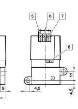
1 Inlet port (G1/8 or 1/8 NPT) 2 Outlet port (G1/8 or 1/8 NPT) 3 Exhaust, do not obstruct 4 Span adjust pot (under lid) **5** Power (3 wire units only) Signal (2 & 3 wire units) Common (2 & 3 wire units) 8 Adjust zero Inlet port (11,1 ID x 1,6 CS O-ring supplied)
