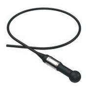
The D/70/H is a true spherical and balanced element combined with a low noise differential pre-amplifier. Signals can be transmitted along cable lengths up to 500m, without any degradation. The pre-amplifier gain options of 20, 30 and 40 dB (are pre-set during manufacture) to suit the customer requirements.
