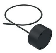
The 395 SERIES transducer is intended for vertical depth sounding applications. The frequencies selected are compatible with a wide range of echo-sounder types. The concentric element arrangement generates a conical beam pattern with low side lobes. The polyurethane housing provides a mechanically robust, corrosion free transducer, suitable for tank, thru-hull or over-side mounting.
