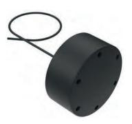
The 65 SERIES transducer is a high power, long range directional array operating at several frequencies. Originally designed for over-side installation, the 65 SERIES can also be hull mounted. The nodal mounted tonpilz elements are extremely robust, capable of withstanding high slamming forces, highly efficient and provide an excellent front to back ratio. An
