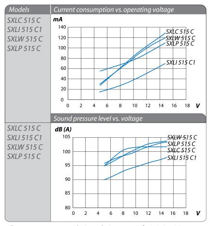
All measurements are made @ 12Vdc @ 1 meter in free air @ 21°C.
