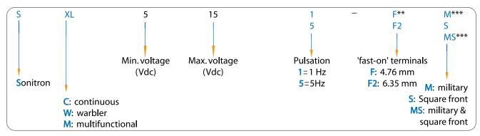
F\*\* If no terminal specification, the model is standard delivered with round pins, diameter 1.5 mm. Fast-on terminals are available in 2 dimensions: F = 4,76 mm (0,187 inch) or F2 = 6,35 mm (0,250 inch).
