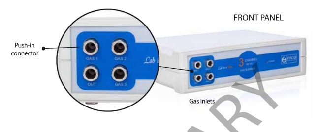
The front panel of the Gas Blender 100 series contains four quick connector for the insertion of input tubes and for the output of the blend. Tubes with an external diameter of 6 mm can be inserted in the push-in connector. MCQ suggest to use tubes made of Tygon/Viton/PTFE/Stainless Steel/Polyurethane.
