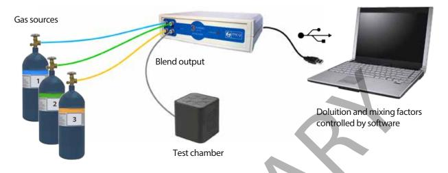
The gas cylinders can be simply connected to the push-in connectors through appropriate tubes, the output of the device must be connected to the test chamber or to the environment for custom applications where the blend is delivered. The mixing and dilution factors can be controlled by software, where the desired flow in each channel can be set and the actual gas flow is continuously displayed in a plot.
