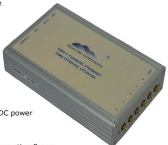
The T680 contains five wide-range time stampers. Each channel can snapshot the time of the rising edge of one electrical input, to 12.2 picosecond resolution with 48 bit range. In timestamp mode, individual time stamps may be read. In TIC mode, channel 0 may be used as the "start" time reference for channels 1-4, with the option to acquire times after or before/after the start event.
