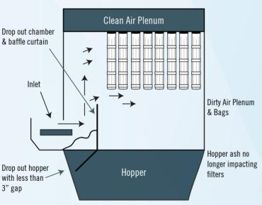
The differential pressure has remained at 30% lower than the conventional filters while the gas flow rate has been maintained equal to that of the conventional filters. There have been no unplanned corrective maintenance entries to remedy filter abrasion and emissions have been maintained below licensed limits.
