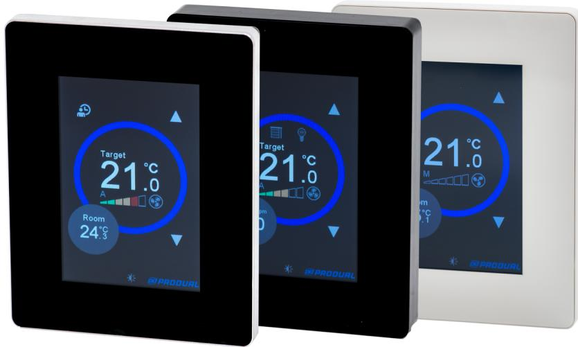
TRC-3A room controllers are designed for climate control in room spaces with modern sharp slim line 3.5" colour touchscreen interface. The controllers have up to two heating and cooling control stages, fan speed control, optional CO<sub>2</sub> level control and humidity control. The units can be in various climate control applications, fan coil units, chilled ceiling and zone heating/cooling systems.
