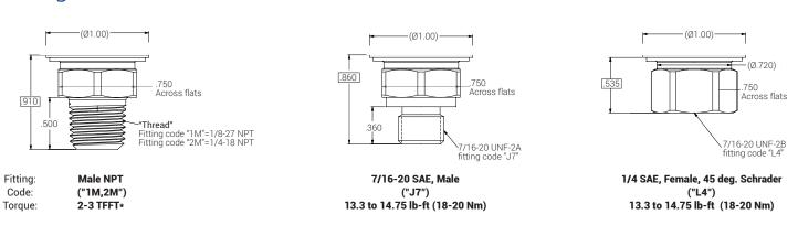
Total height= Electrical termination height + Housing height + Fitting connection height (dimensions boxed above)
