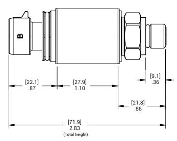
\*Shown with 7/16" SAE Ext. fitting (J7) and 3 Pin Packard termination (P1).
