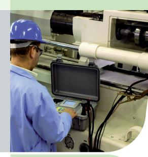
MI 3252 MicroOhm 100A is a portable low resistance ohmmeter used to measure low contact resistances of breakers and switches, busbars using test current from 100 mA to 100 A.
