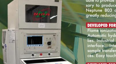
able to provide a residual solvent result in the time necessary to produce a single roll (12 minutes). The use of Neptune 803 allows process corrections in real time, greatly reducing waste and rework of products.
