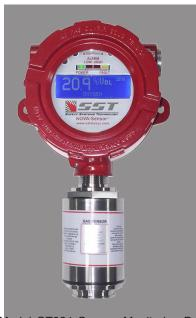
The SST Model GT824 Oxygen Monitoring Detector is a completely self-contained device that measures and displays the concentration of oxygen present in a protected area, performs local control functions, and optionally transmits this information to a central control point. Two alarm relays and a fault relay are included.
