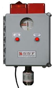
The SST Model GT823 includes a high reliability microprocessor based transmitter/controller in a compact, one piece construction. Just mount, apply power and you have a complete monitoring and notification of low or high oxygen concentrations. A digital readout continuously displays operting status and the actual concentration of oxygen.
