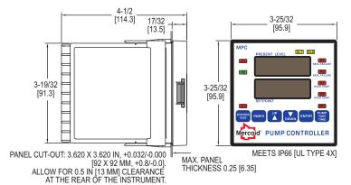
The Series MPC Pump Controller provides versatile level control in a standard 1/4 DIN package. Designed for use with almost any style level transmitter the unit displays the present level and main set point value. Incorporated in the MPC is programmable level differential for on/off control of one or two pumps, valves, or other devices through two SPDT relays.
