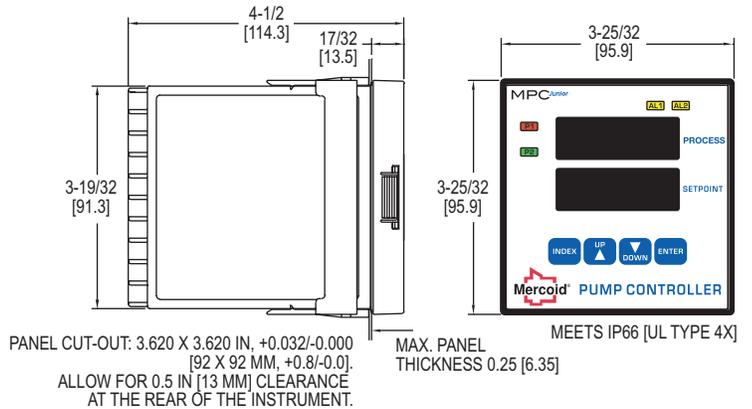
The **Series MPC JR Pump Controller** provides versatile level control in a standard 1/4 DIN package. Designed for use with almost any style level transmitter the unit displays the present level and main set point value. Incorporated in the MPC JR is programmable level differential for on/off control of one or two pumps, valves, or other devices through two SPDT relays.
