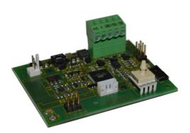
Digital interface compatible to all smartGAS EVO – sensors: BASIC<sup>EVO</sup> FLOW<sup>EVO</sup>
